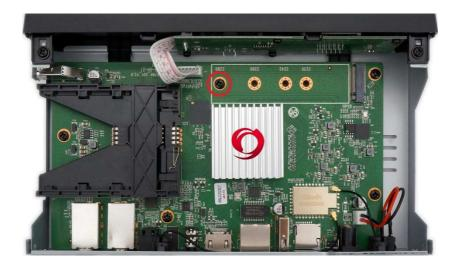
Insert the M. 2 SSD at a 30-degree angle into the appropriate slot. Press the
